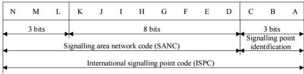
Gambar II. 4 Format *International Signalling Point Code (ISPC)*
